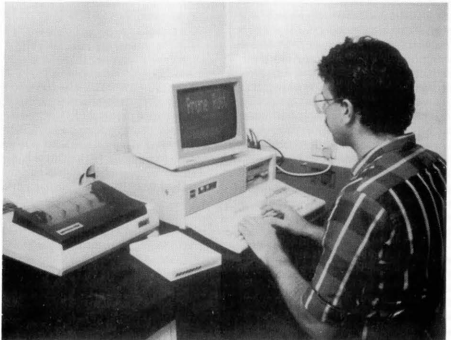
Figure 3. A personal computer being used to obtain potential infection period data from a remote Prune Rust Infection Predictor (PRIP). Horticultural advisors access PRIP units located in orchards via telephone connections. Software developed for the application allows the advisors to evaluate the potential rust infection and to obtain a prognosis of likely seasonal severity of the disease. This permits rapid issuing of warnings to farmers. (Photo: L. Turton).
